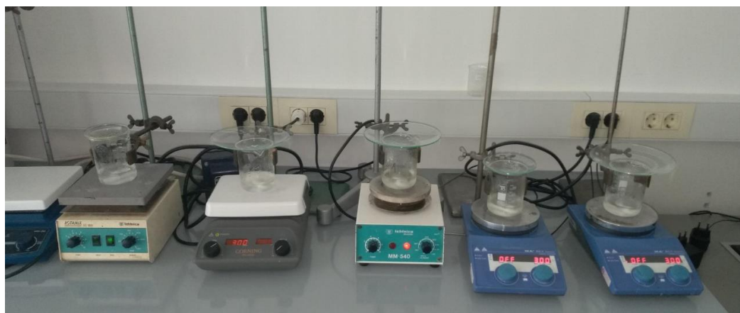
Figure 10. Stirring of PEO/NaAlg liquid mixture on the magnetic stirrer
