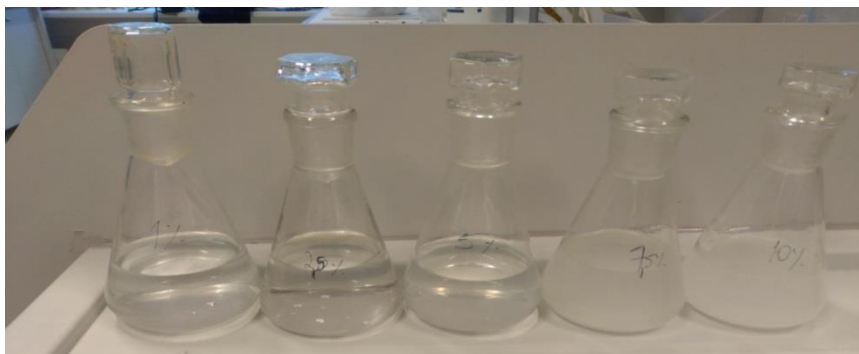
Figure 14. Different solutions of CaCl 2 in methanol
