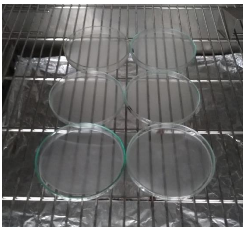
Figure 12. Polymer films after 48 hours of drying in oven
