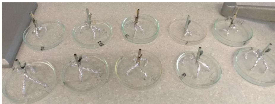
Figure 15. Immersion of 80%PEO/20%NaAlg films in \text{CaCl}_2 solutions
