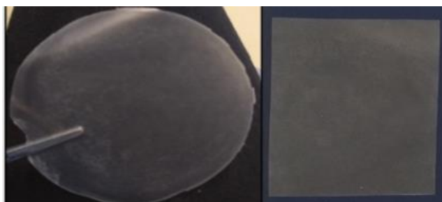
Figure 13. 80%PEO/20%NaAlg film after five days of drying and after cutting in wanted shape
