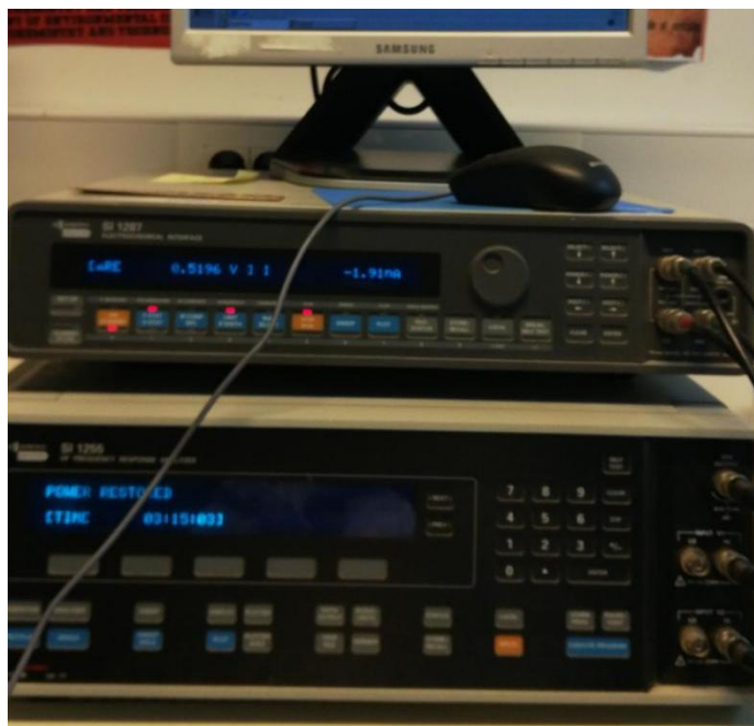
Slika 11. Potenciostat/galvanostat "Solartron SI 1287" i "Solartron HF Frequency Response Analyzer (FRA) SI 1255".
