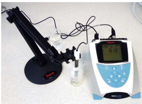
Slika 2.2. pH-metar Orion 4 STAR Thermo Scientific.
