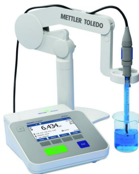
Slika 19. pH metar Seven Multi firme Mettler Toledo
