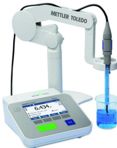
Slika 19. pH metar Seven Multi firme Mettler Toledo
