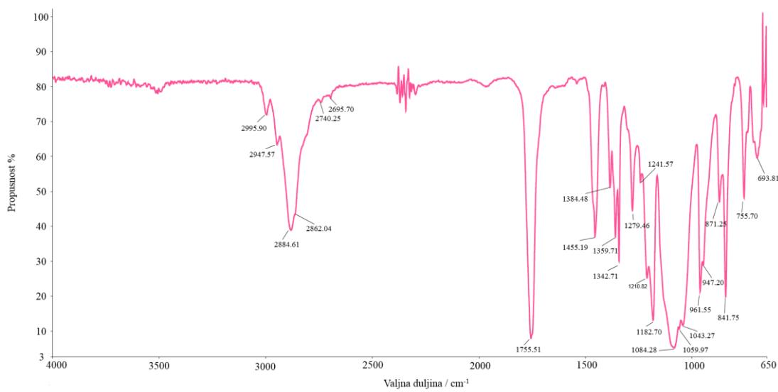
**Slika 30.** FTIR spektrogram mješavine PLA/PEO (50/50)
