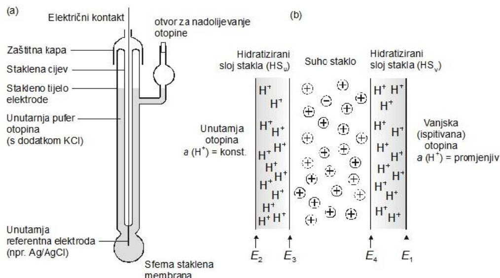
**Slika 9.** Prikaz staklene elektrode (a) i presjek kroz staklenu membranu (b)<sup>3</sup>
