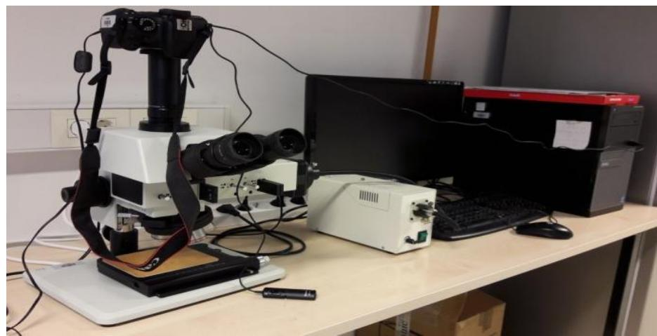
**Slika 17.** Optički mikroskop MXFMS-BD, Ningbo Sunny Instruments Co.
