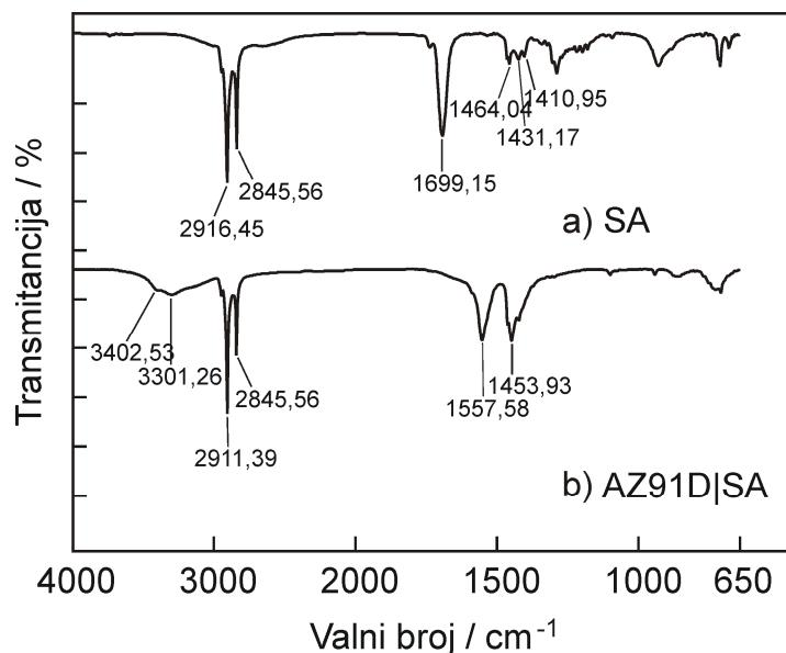
**Slika 4.16.** (a) FTIR spektar praha SA i (b) FTIR spektar AZ91D legure modificirane SAMom SA.
