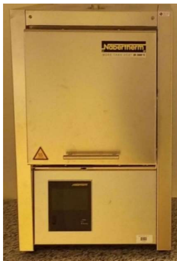
Slika 13. Visokotemperaturna peć, Nabertherm LTH 04/18.
