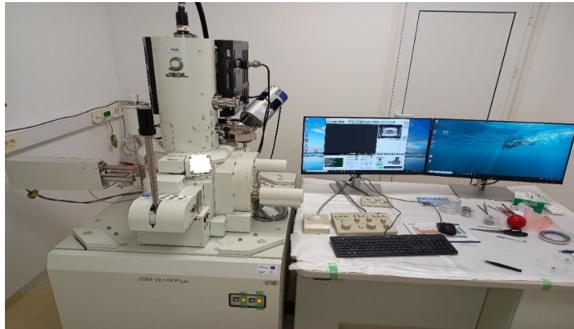
Slika 27. JSM-7610FPlus Schottky Field Emission Scanning Electron Microscope
