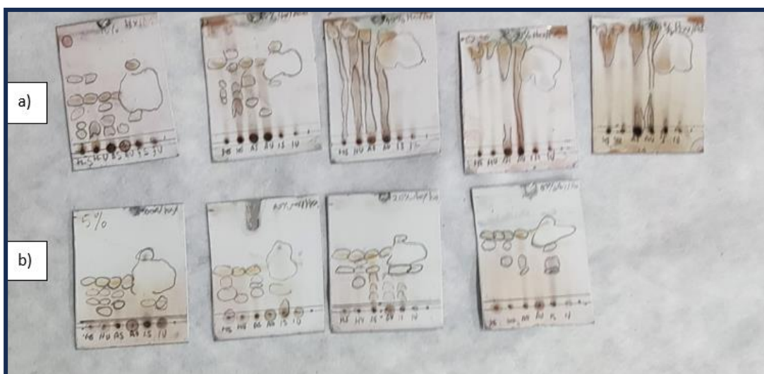
Figure 27. TLC plates of the solvent systems, a) hexane/ethyl acetate, b) hexane/acetone. HexS: hexane Soxhlet; HexU: hexane ultrasound; AceS: acetone Soxhlet; AceU: acetone ultrasound; iPrOHS: isopropanol Soxhlet; iPrOHU: isopropanol ultrasound
