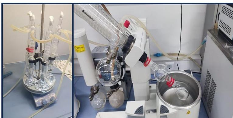
**Figure 25.** Soxhlet extraction system of *S. glabrum* (left), rotary evaporator (right)
