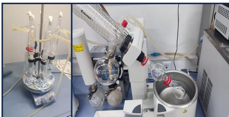
Figure 25. Soxhlet extraction system of S. glabrum (left), rotary evaporator (right)
