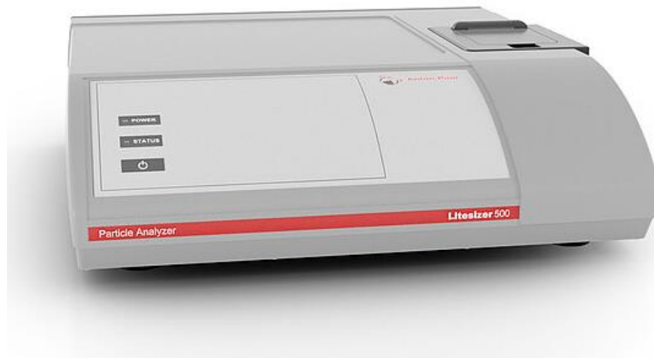
Slika 16. Instrument DLS Litesizer 500 Anton Paar
