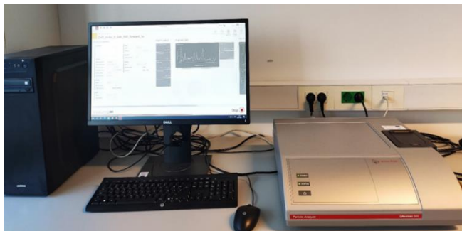
Slika 20. Particle size Analyzer: Litesizer 500, Anton Paar
