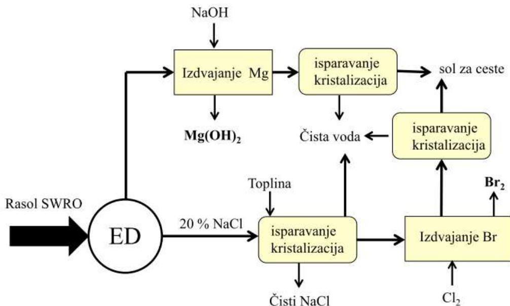
Slika 15. Dijagram toka obrade rasola SWRO s ED i izdvajanje  $\text{NaCl}$ ,  $\text{Br}_2$  i  $\text{Mg}(\text{OH})_2$ <sup>5</sup>
