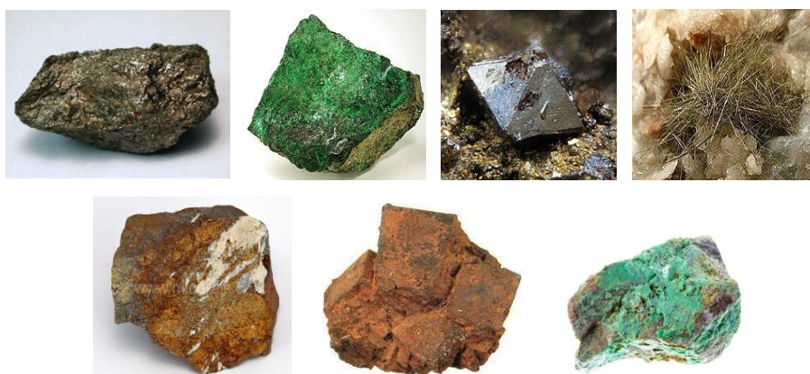
Slika 1. Neki primjeri niklovih ruda: 1 – pentlandit, željezo-nikal sulfid, (\text{Fe,Ni})_9\text{S}_8 . 2 - hazlevudit, \text{Ni}_{1,5}\text{S} , \text{Ni}_{17}\text{S}_{18} , \text{Ni}_3\text{S}_2 , 3 – polidimit, \text{Ni}_3\text{S}_4 , 4 - milerit, \text{NiS} , 5 – nikelin, \text{NiAs} , 6 – limonit, (\text{Fe,Ni})\text{O}(\text{OH}) , 7 – garnierit, vodenasti niklov silikat (\text{Ni,Mg})_3\text{Si}_2\text{O}_5(\text{OH})_4 . [1]
