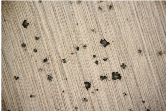
Figure 34 Optical micrographs for the AISI 304L after potentiodynamic polarization measurements in seawater at 15°C (magnification 100 times).
