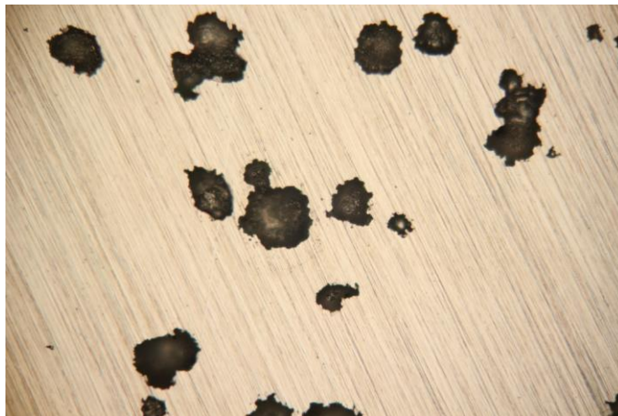
Figure 35 Optical micrographs for the AISI 304L after potentiodynamic polarization measurements in seawater at 25°C (magnification 100 times).
