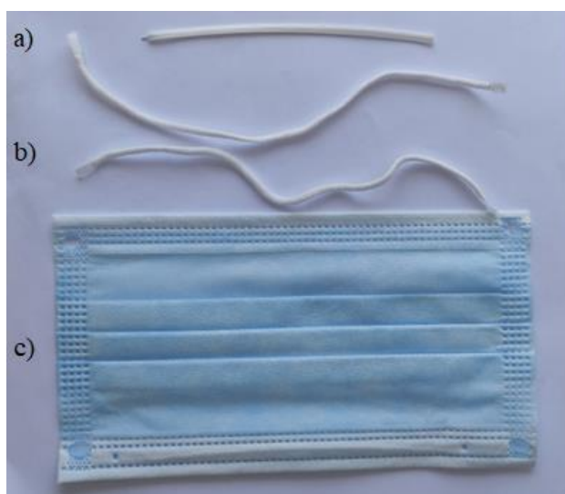
Figure 17. Single-use face mask components – a) metal material, b) ear loop, c) face filter
