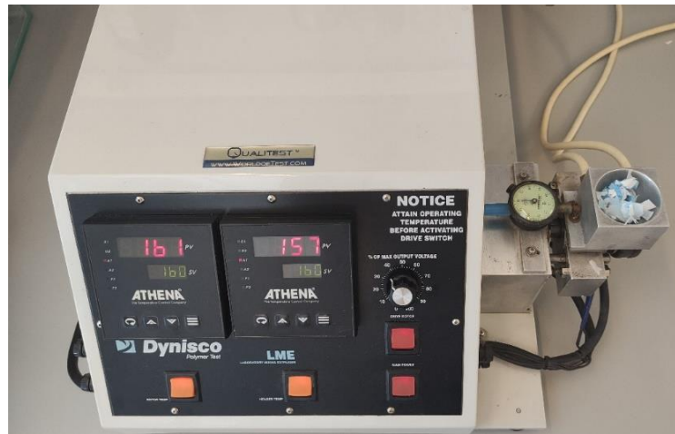
Figure 19. Laboratory single-screw extruder Dynisco (Qualitest, USA)
