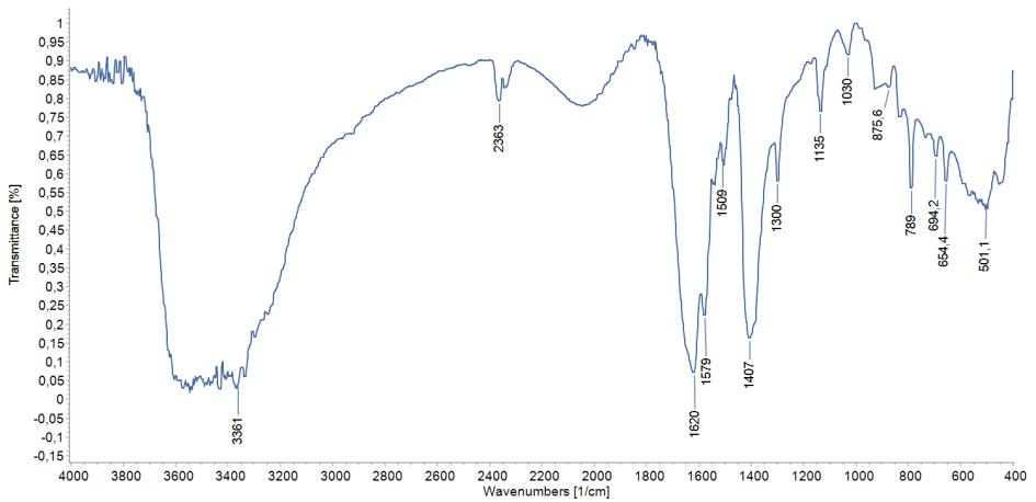
*Slika 5.* IR spektar  $[\text{Cu}(6\text{-OHnic})_2(\text{H}_2\text{O})_2]$  za  $\text{pH} = 6$
