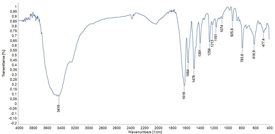
*Slika 4.* IR spektar  $[\text{Cu}(2\text{-OHnic})_2(\text{H}_2\text{O})_2]$  za  $\text{pH} = 6$
