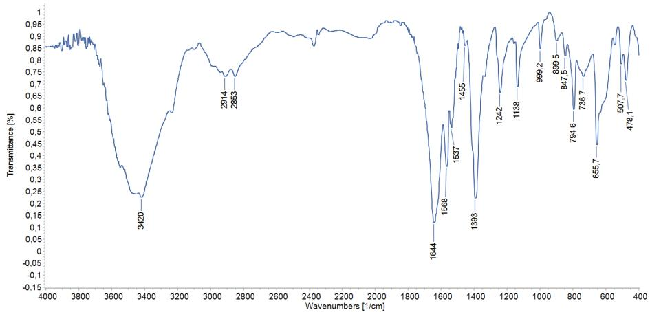
*Slika 2.* IR spektar  $[\text{Co}(\text{H}_2\text{O})_6](6\text{-OHnic})_2$
