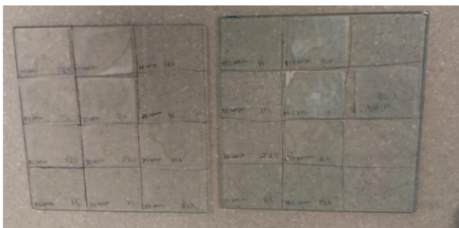
Figure 16. The blend films after cross-linkage and rinsing with methanol
