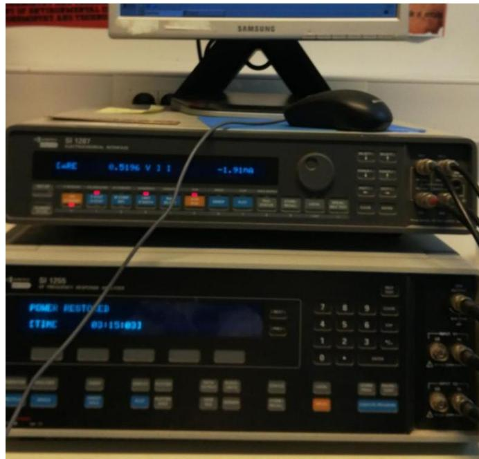
**Slika 11.** Potencijostat/galvanostat "Solartron SI 1287" i "Solartron HF Frequency Response Analyzer (FRA) SI 1255".
