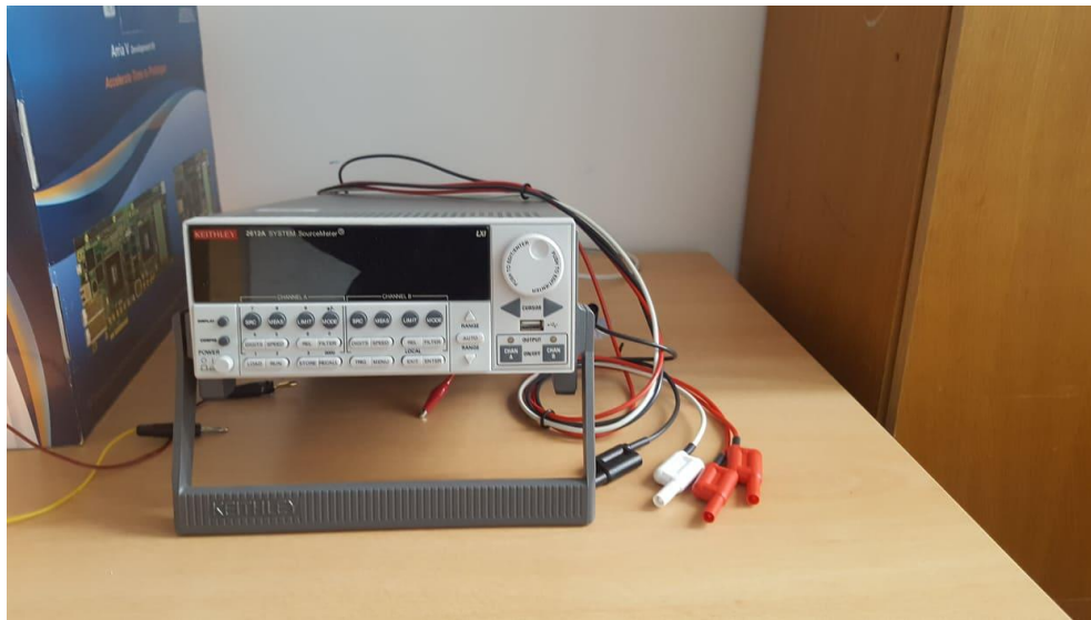
Slika 2.2. Keithley 2612A Source-Measure-Unit
