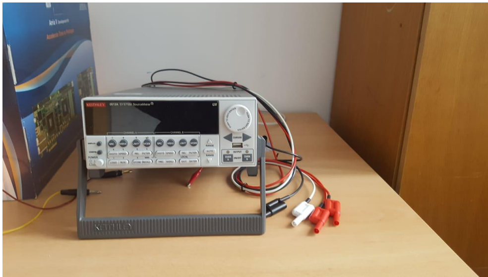
Slika 2.2. Keithley 2612A Source-Measure-Unit
