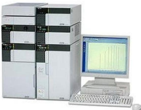
**Slika 6.** HPLC LC-20 series, Shimadzu
