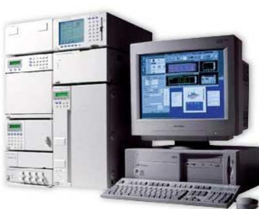
**Slika 5.** HPLC LC-10 series, Shimadzu
