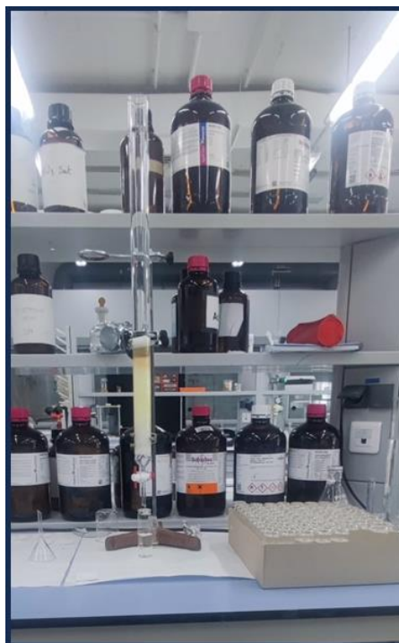
Figure 28. The column chromatography system
