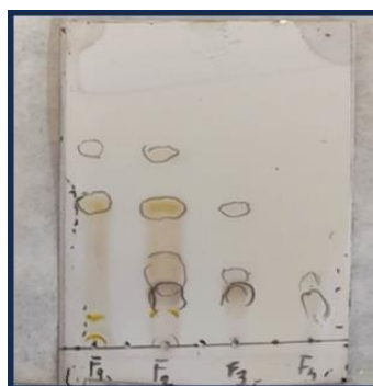
Figure 31. TLC analysis of the column chromatography of subfractions F 3.2 and F 3.3
