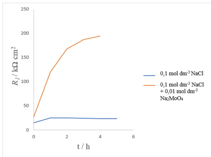
**Slika 4.2.** Ovisnost otpora  $R_1$  o vremenu, tijekom boravka Sn elektrode u  $0,1 \text{ mol dm}^{-3}$  otopini NaCl i u  $0,01 \text{ mol dm}^{-3}$  otopini  $\text{Na}_2\text{MoO}_4$  u  $0,1 \text{ mol dm}^{-3}$  otopini NaCl.
