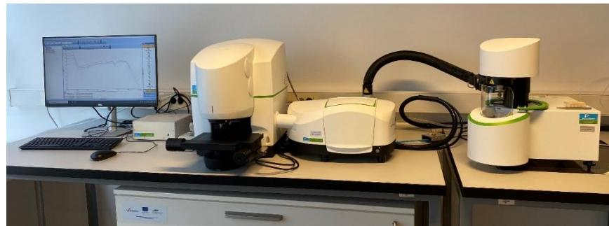
**Slika 16.** FT-IR spektrometar Spectrum Two, Perkin Elmer
