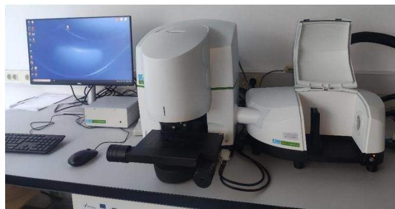
**Slika 12.** FT-IR spektrometar Spectrum Two, Perkin Elmer
