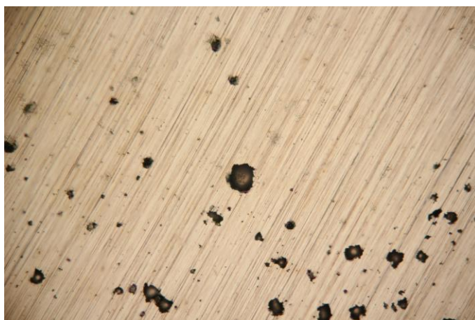
Figure 41 Optical micrographs for the AISI 316L after potentiodynamic polarization measurements in seawater in the presence of 10 ppm of S 2- at 25°C (magnification 100 times).
