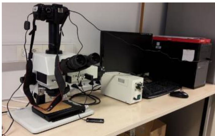
Figure 20 Light microscope MXFMS-BD Ningbo Sunny Instruments co. 48
