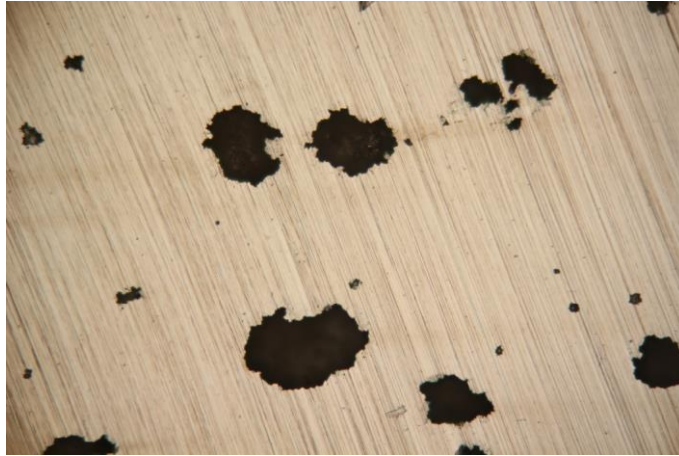
Figure 36 Optical micrographs for the AISI 304L after potentiodynamic polarization measurements in seawater at 35°C (magnification 100 times).
