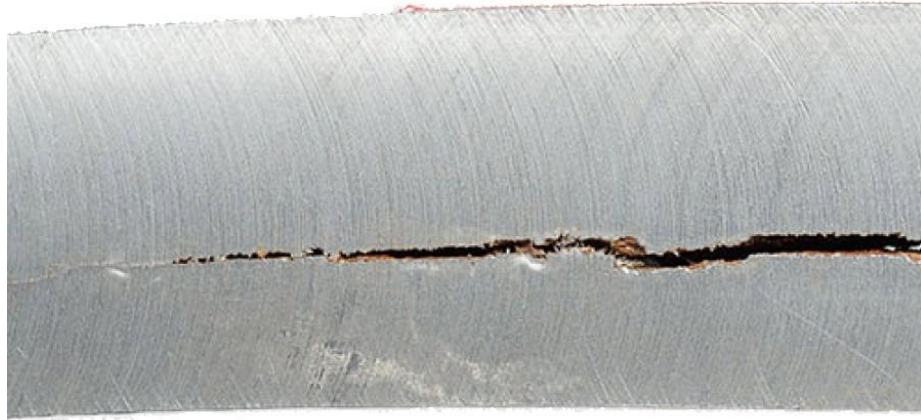
Figure 17 Stress corrosion cracking in stainless steel. 46
