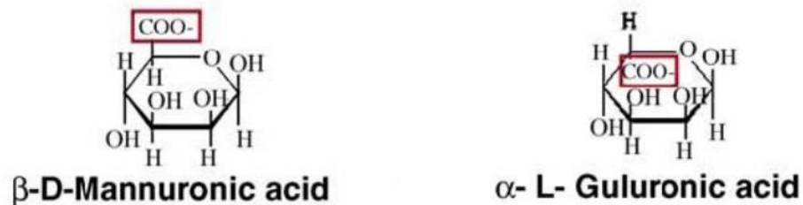
Figure 6. Molecular structure of \beta -D-mannuronic acid and \alpha -L-guluronic acid
