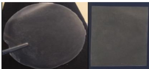
Figure 13. 80%PEO/20%NaAlg film after five days of drying and after cutting in wanted shape
