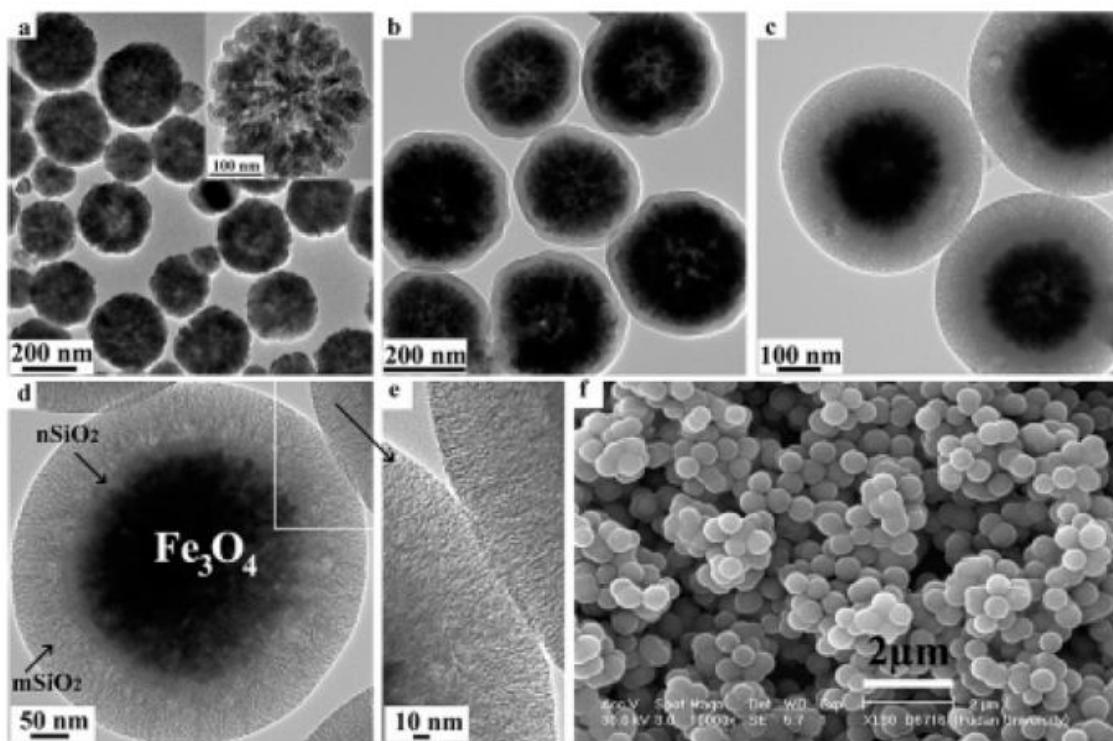
**Slika 7.** TEM slike (a)  $\text{Fe}_3\text{O}_4$  čestica, (b)  $\text{Fe}_3\text{O}_4/\text{nSiO}_2$ , (c-e)  $\text{Fe}_3\text{O}_4/\text{nSiO}_2/\text{mSiO}_2$  mikrosfera i (f) SEM slika  $\text{Fe}_3\text{O}_4/\text{nSiO}_2/\text{mSiO}_2$  mikrosfera.<sup>2</sup>
