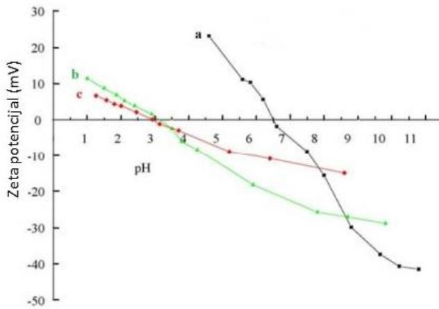
Slika 16. Zeta potencijal  $\text{Fe}_3\text{O}_4$  nanočestice (a),  $\text{Fe}_3\text{O}_4/\text{SiO}_2$  nanočestice (b) i  $\text{SiO}_2$  (c).<sup>2</sup>
