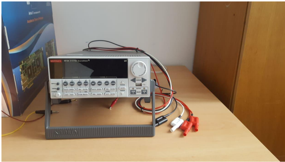
Slika 2.2. Keithley 2612A Source-Measure-Unit
