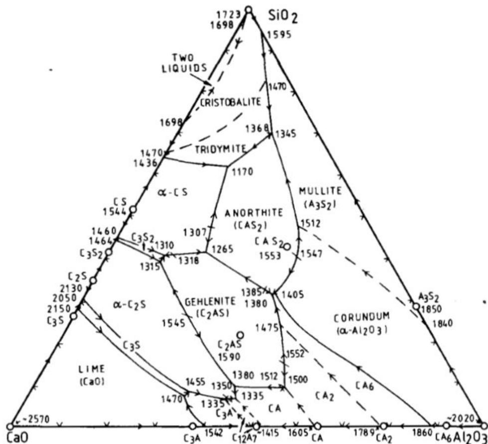
**Slika 6.** Sustav CaO-Al<sub>2</sub>O<sub>3</sub>-SiO<sub>2</sub>. [11]
