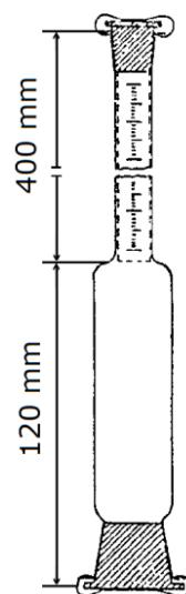
Slika 6. Volumenometar<sup>1</sup>
