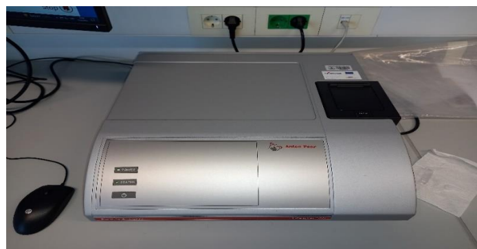
Slika 28. Dynamic Light Scattering Litesizer 500
