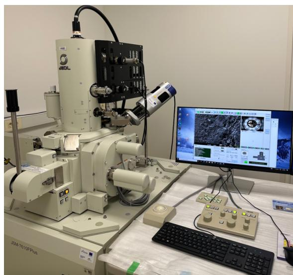
Slika 17. SEM/EDS JEOL JSM – 7610F Plus.
