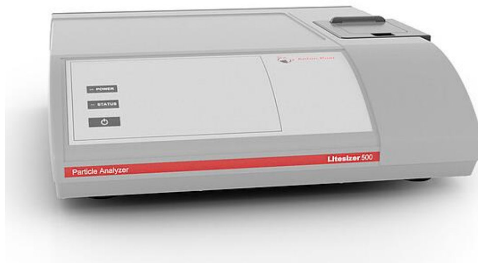
Slika 16. Instrument DLS Litesizer 500 Anton Paar
