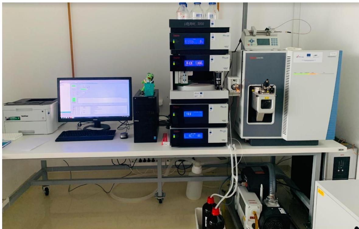
Slika 15. UHPLC-DAD-MS/MS instrument
