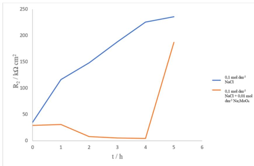
**Slika 4.4.** Ovisnost otpora  $R_2$  o vremenu, tijekom boravka Sn elektrode u  $0,1 \text{ mol dm}^{-3}$  otopini  $\text{NaCl}$  i u  $0,01 \text{ mol dm}^{-3}$  otopini  $\text{Na}_2\text{MoO}_4$  u  $0,1 \text{ mol dm}^{-3}$  otopini  $\text{NaCl}$ .
