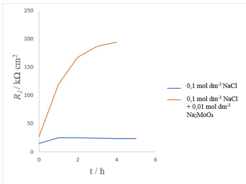
**Slika 4.2.** Ovisnost otpora  $R_I$  o vremenu, tijekom boravka Sn elektrode u  $0,1 \text{ mol dm}^{-3}$  otopini NaCl i u  $0,01 \text{ mol dm}^{-3}$  otopini  $\text{Na}_2\text{MoO}_4$  u  $0,1 \text{ mol dm}^{-3}$  otopini NaCl.
