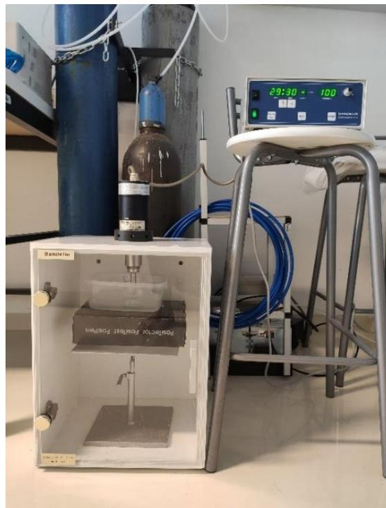
**Slika 16.** Ultrazvučna sonda (Ultrasonic homogeniser, Bandelin HD 2200, 20 kHz, 200 W)
