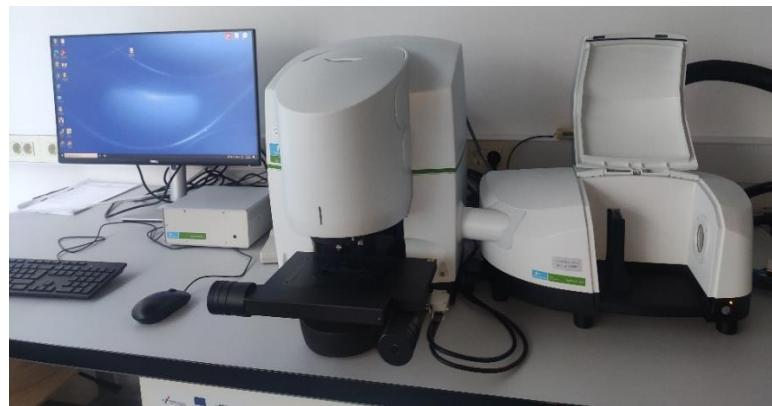
**Slika 22.** FT-IR spektrometar Spectrum Two, Perkin Elmer
