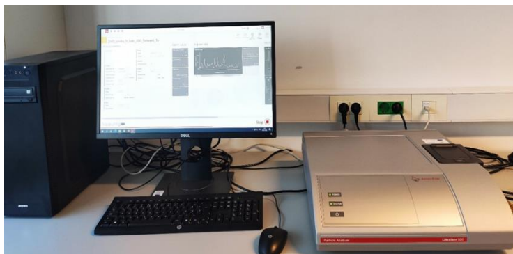
Slika 20. Particle size Analyzer: Litesizer 500, Anton Paar
