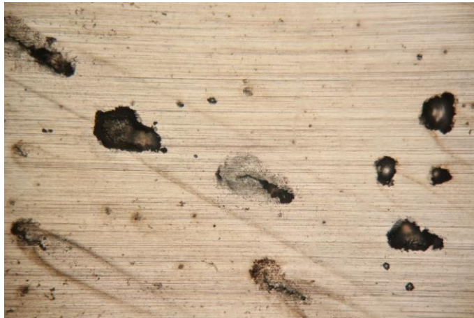
Figure 40 Optical micrographs for the AISI 304L after potentiodynamic polarization measurements in seawater in the presence of 10 ppm of S 2- at 25°C (magnification 100 times).
