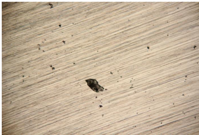
Figure 37 Optical micrographs for the AISI 316L after potentiodynamic polarization measurements in seawater at 15°C (magnification 100 times).
