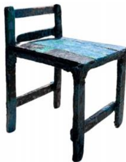
Figure 13. Kids chair produced from recycled polypropylene face masks (filter layer and ear loop) 1
